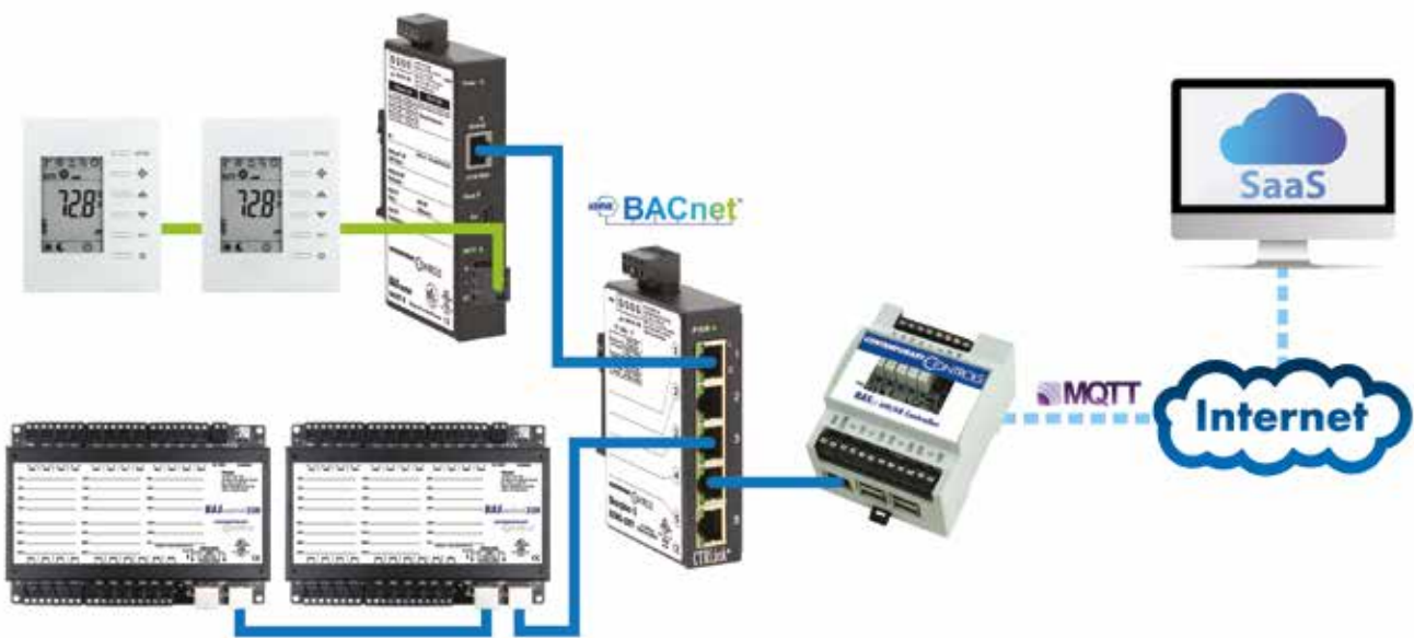
Figure 1: A Cloud-Connected BACnet Controller Uses SaaS to Exchange Data Over the Internet.
